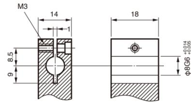
Tightening torque: 0.6 N·m
