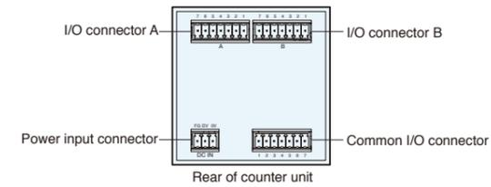
Use a shielded cable for connection to the FG pin on the rear of the counter unit. (Prepare a shield cable by yourself.)
