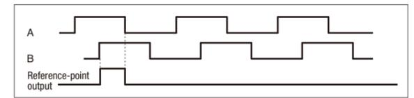
The reference point is synchronized with A and B phases at high impedance. (Note: this may not be worded correctly)
