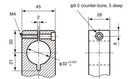
Tightening torque: 6 N·m
