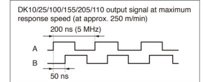
The A/B quadrature output signal by measuring unit is 5 MHz maximum with a minimum phase difference of 50 ns for DK800SA and is 2.5 MHz maximum with a minimum phase difference of 100 ns for DK800SB.
