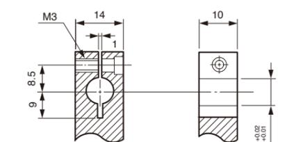
Tightening torque: 0.18 to 0.23 N·m
