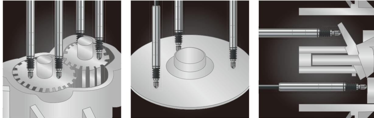
Assembled part measurement and shim selection
