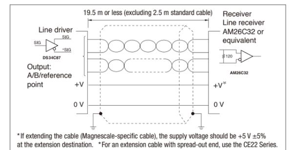
\*If extending the cable (Magnescale-specific cable), the supply voltage should be +5 V  $\pm$ 5% at the extension destination. \*For an extension cable with spread-out end, use the CE22 Series.
