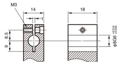
Tightening torque: 0.6 N·m
