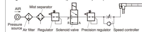
Fig. 2 Pneumatic circuit (vacuum suction)
