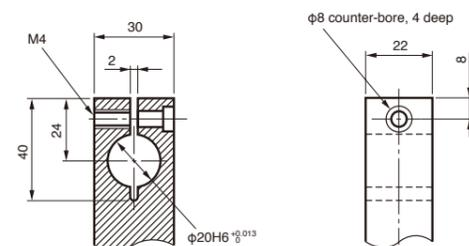
Tightening torque: 4 N·m
